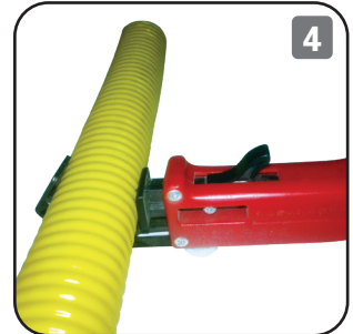
Cutting the hose by apparatus and undressing the outer coating. Can the coating be undressed first, then the cutting shall also be performed.
