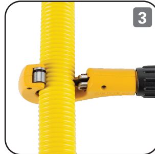
The hose should only be cut 360 degrees using the cutting apparatus. It should not be torn off by hand. Cut stone etc. should not be used.
